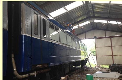
**Class 121 55029:** The Rushden bubble continues to progress with more of the fie damaged bodyside cleaned up and repainted. Varnished indicator boxes have also been completed.
